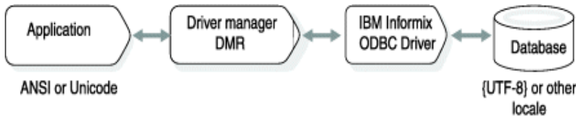
Figure 8. Typical ODBC application architecture
