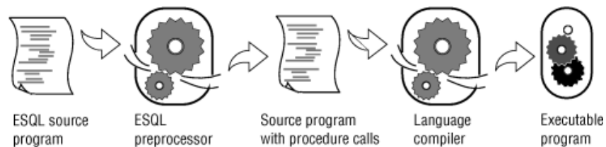
Figure 367. Overview of processing a program with embedded SQL statements
