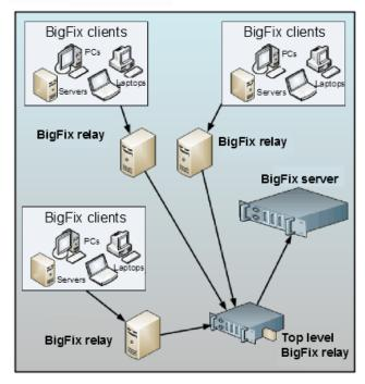
This diagram displays a typical data center layout, where there are between 1,000 and 10,000 endpoints in the data center.
