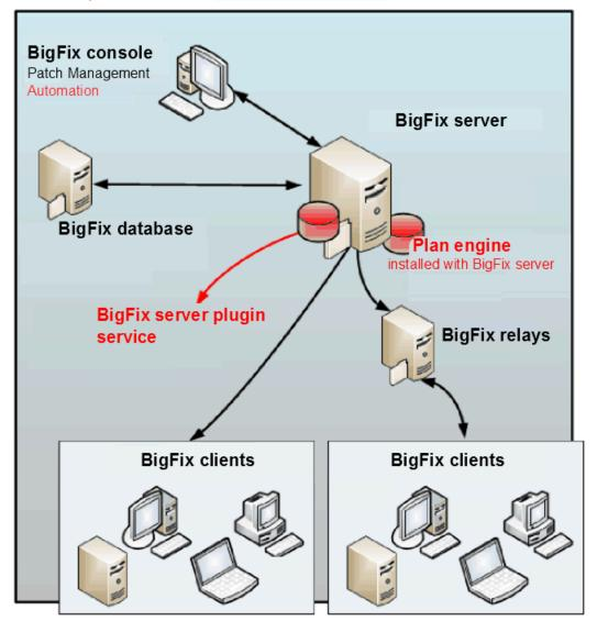
The Automation Plan Engine communicates with the BigFix server via the REST API. The BES server plugin service is required on the BigFix server. Server Automation requires no additional components. Server Automation can operate with or without relays.
