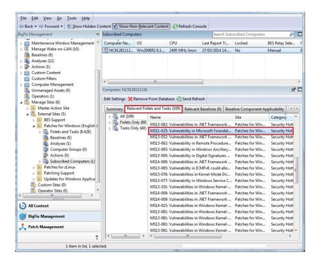
A Fixlet is relevant for a client if the client needs to install the content referenced in the Fixlet. The need to install that content is automatically evaluated on the Client using a set of predefined conditions specified in Fixlet.
