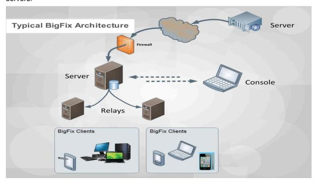
The console oversees this activity. It connects to the server and periodically updates its views to reflect changes or new information about your network. When vulnerabilities are discovered, the console operator can target patches or other fixes to the appropriate computers. The progress of the fixes can be followed in near real time as they spread to all the relevant computers and, one by one, eliminate bugs and vulnerabilities.
