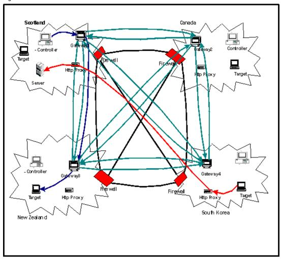
In this scenario the targets and controllers are distributed over several locations, all of which are protected by a firewall. The firewalls prevent the controllers from connecting directly to the target in remote locations, but they do allow the gateways to connect to *gateways and gateways only*, in remote locations. The existing HTTP Proxy servers, allow the targets to connect to the server.
