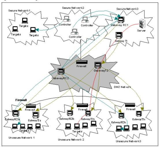
In this scenario there are two well defined networks, a secure network where the server is installed and the controllers machines are located and an unsecure network, it could be a web facing network, where servers need to be accessed for maintenance and problem resolution.
